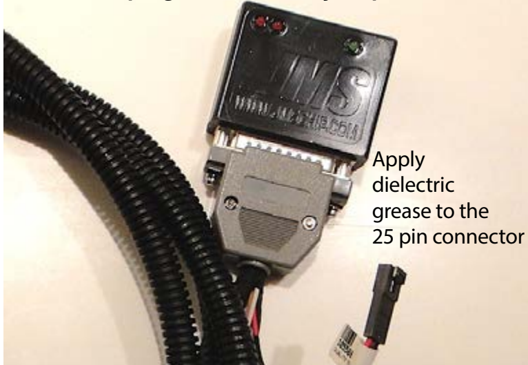
BoostMAX plugs into the Grey 25 pin connector
